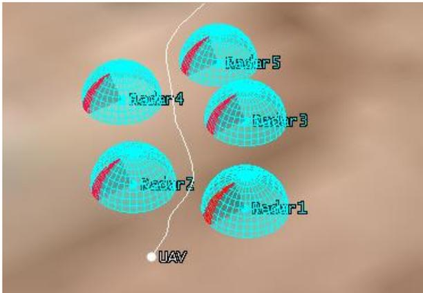
**Figure 5:** Propagated Route for UAV on STK using the Optimal Points Computed by A\* Algorithm
