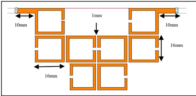
Fig.5 Layout of the eight-pole microstrip band-pass filter on  $\epsilon_r = 4.4$  and  $h = 1.6$  mm.
