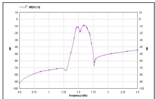
Fig.4 Full-wave EM simulated insertion loss response of the filter for  $\epsilon_r = 4.4$  and  $h = 1.6$ .
