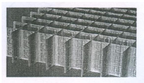
Fig.1 Metamaterial Proposed by D.R. Smit
