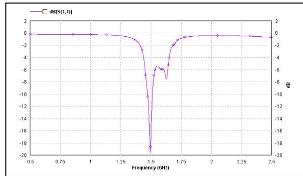
Fig.3 Full-wave EM simulated return loss response of the filter for  $\epsilon_r = 4.4$  and  $h = 1.6$ .
