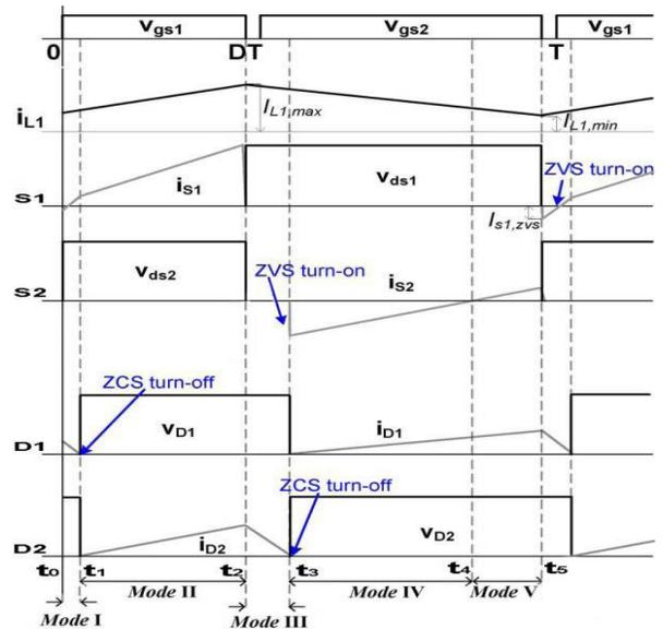
Fig 2: Key waveforms for soft switched boost converter
