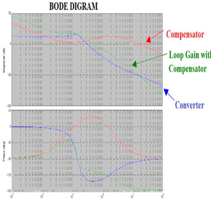
Fig 4: Bode plot of open loop(blue), compensator(red) and loop gain(green)
