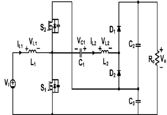
Fig 1: Soft switched boost converter
