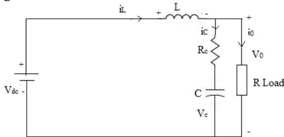
Fig. 2 Equivalent circuit when switches  $S_1$  and  $S_2$  are ON.
