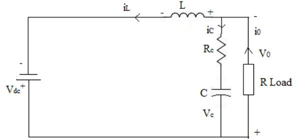
Fig. 3 Equivalent circuit when switches  $S_3$  and  $S_4$  are ON
