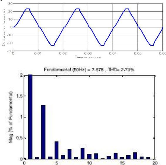
Fig. 7 Simulation Result of PR controller
