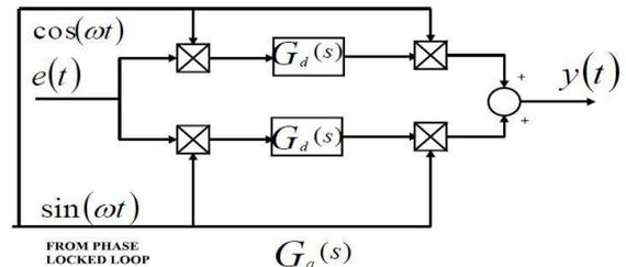
Fig. 6 Single phase equivalent presentation of PR controller
