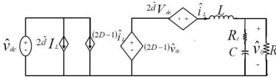
Fig. 4 Small signal model of 1-Φ inverter
