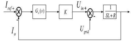
Fig. 5 System Model with PI control
