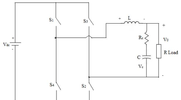
Fig. 1 Schematic diagram of grid-connected inverter
