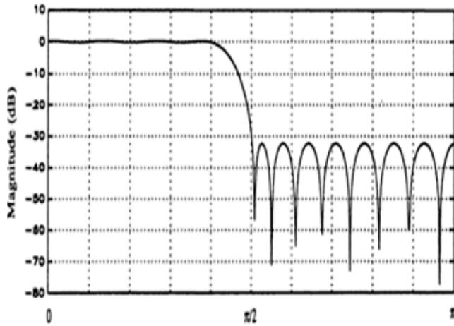
Fig.4 Frequency Response for Equiripple FIR filter
