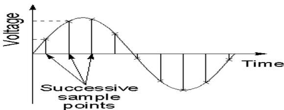
Fig. 1 Waveform sampling for Digital Signal Processing.
