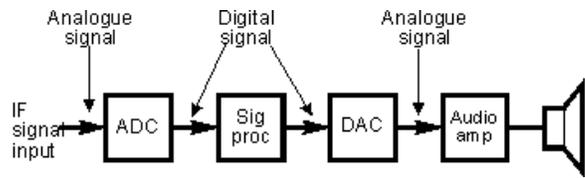
Fig.2 Digital Signal Processor block diagram.
