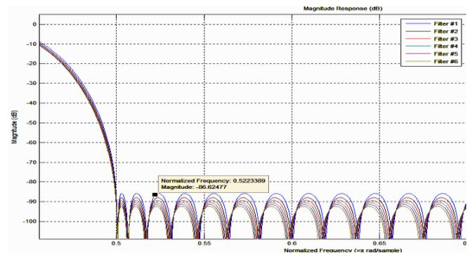
Fig.6 Stop Band Attenuation for Different weights.
