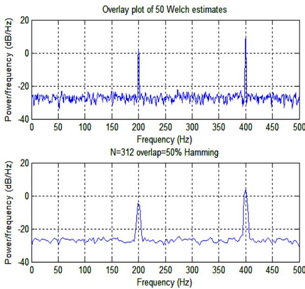
Fig. 2. Data sequence in Hamming window
